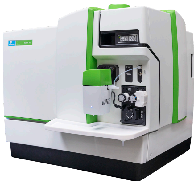
Figure 2. SampleSense prepFAST integrated with NexION 2000 ICPMS.
